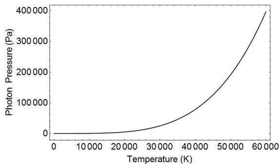
**Figure 1. Photon pressure as a function of temperature in vacuum. Photon pressure is calculated for the volume of  $V = 2.47 \times 10^{-2} \text{m}^3$ . Photon pressure is 1 bar at  $T = 42515 \text{K}$  in vacuum.**
