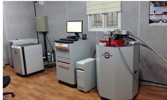
Figure 3. Physical Property Measurement System (PPMS).
