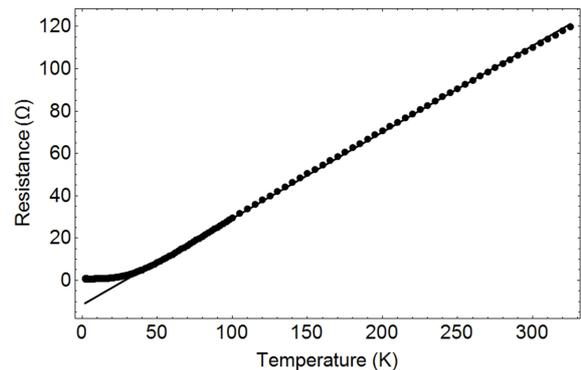
Figure 4. Resistance measurement as a function of temperature for Pt100. The resistance is fitted with  $R = -11.553 + 0.408T$ . The Pt100 shows the linear dependence with temperature for 40K-325 K. Impurity and non-crystal structure can cause the finite resistance as temperature goes down below 40 K.
