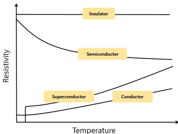
**Figure 2. Cartoon of the resistivity of material types as a function of temperature.**
