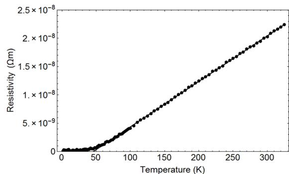
Figure 5. Resistivity measurement as a function of temperature for copper wire. The resistivity of the copper wire shows the linear dependence with temperature for 50K-325 K. Electron-phonon scattering is decreased linearly as temperature decreases. The Cu wire has the diameter of 0.33 mm and the RRR of the copper wire is 126.
