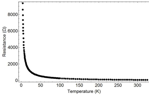
**Figure 6. Resistance measurement as a function of temperature for Cernox sensor. The resistance is increased as temperature decreases.**
