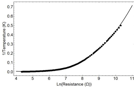
**Figure 7. Theoretical fitting for the resistance measurement of Cernox sensor. The data is fitted with  $\frac{1}{T} = -0.1443 + 0.1178 \ln(R) - 0.0293(\ln(R))^2 + 0.0023(\ln(R))^3$  and this fitting works well.**
