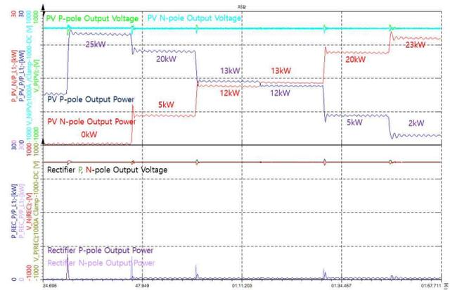
**Fig. 9.** Micro-grid voltage stabilization by independent voltage control of P and N-poles of the PV simulator in the two-pole load simultaneous variation (including mono-pole operation)
