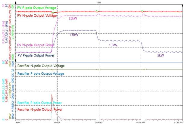
(a) Load variation in P-pole and fixed load in N-pole
