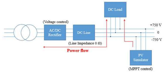
(a) Case 1: Conventional MPPT control of the PV simulator
