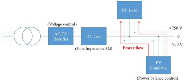
(b) Case 2: Power balance control by the PV simulator
