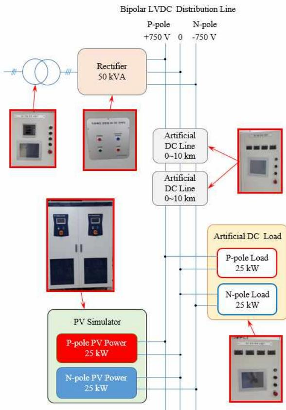
Fig. 1. Configuration of the Experimental set-up
