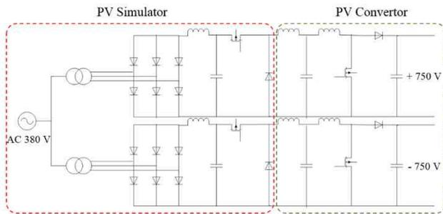
**Fig. 3.** Circuits of PV simulator and converter used in the experiments
