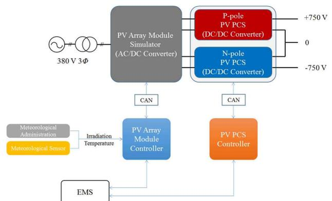
Fig. 2. Block diagram of the PV simulation system developed for bipolar LVDC distribution grid
