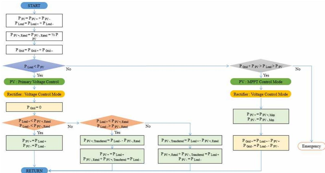
Fig. 6. Flowchart of the power balance control between poles
