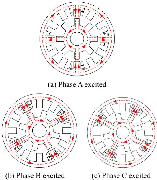
Fig. 2. Flux paths in conventional 12/8 SRM
