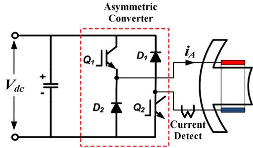
Fig. 15. Topology of asymmetric converter
