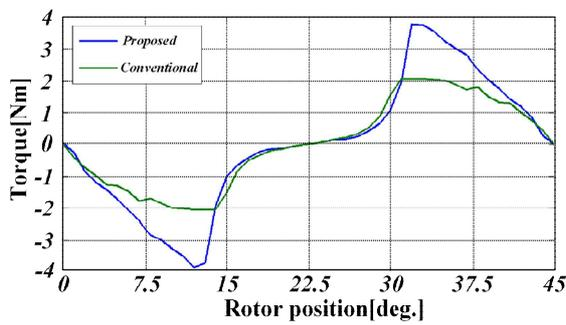
Fig. 10. Torque characteristics of conventional and segmental type SRMs
