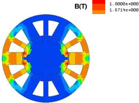
Fig. 8. Magnetic flux density of segmental 12/8 SRM
