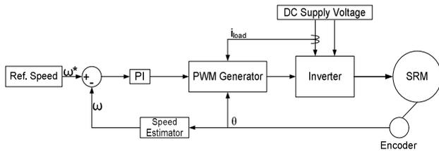
Fig. 18. Control scheme for conventional and segmental
