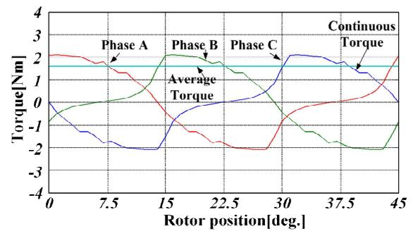
Fig. 11. Continuous torque of conventional type
