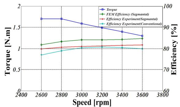
Fig. 19. Efficiency comparisons of conventional and segmental type SRMs
