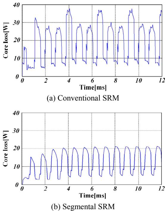
Fig. 17. Core loss profiles at rated condition
