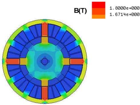
Fig. 7. Magnetic flux density of conventional 12/8 SRM
