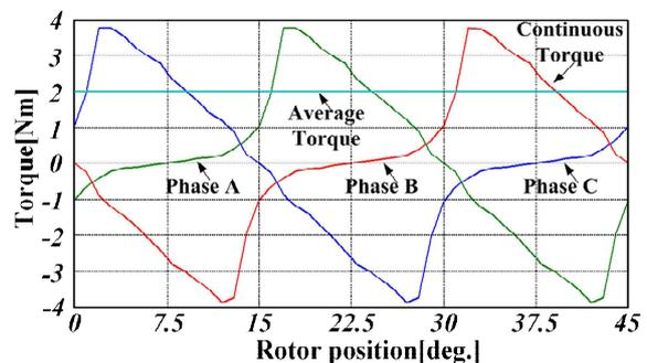
Fig. 12. Continuous torque of segmental rotor type
