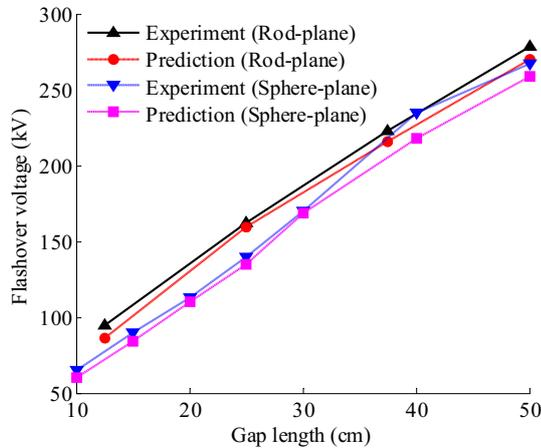
**Fig. 7.** Comparison of the flashover voltage prediction results of rod-plane and sphere-plane gaps with the experimental data
