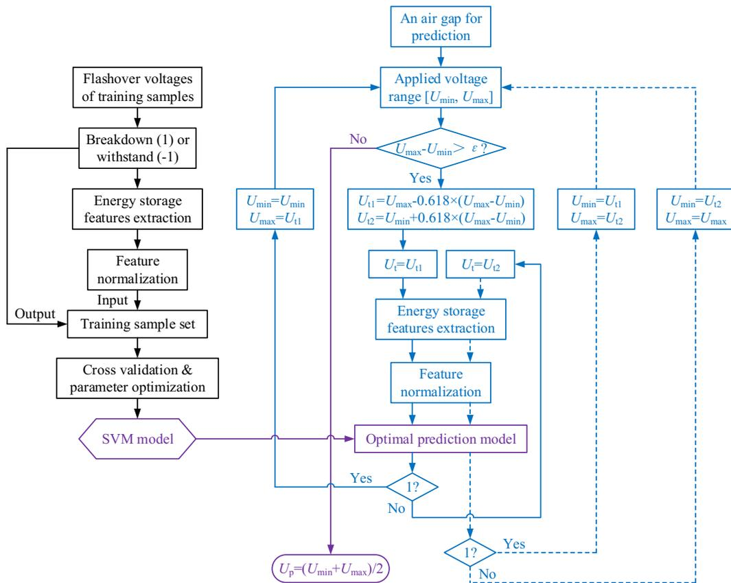
Fig. 2. General flow chart of the prediction method
