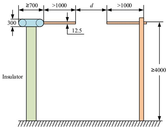
Fig. 3. Arrangement of the standard rod-rod gap (all dimensions are in millimeters)
