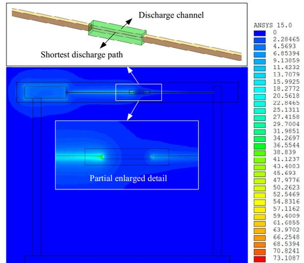
Fig. 4. The electric field distribution of the standard rod-rod gap ( $d=30$  cm) and the schematic diagram of the discharge channel and the shortest discharge path
