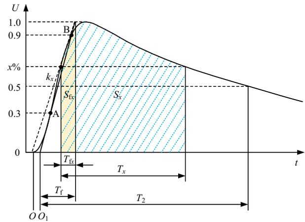
Fig. 1. Definitions of partial impulse voltage waveform features
