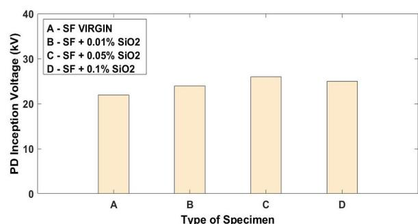
Fig. 2. Partial Discharge Inception Voltage values for virgin and nano modified sunflower oil samples
