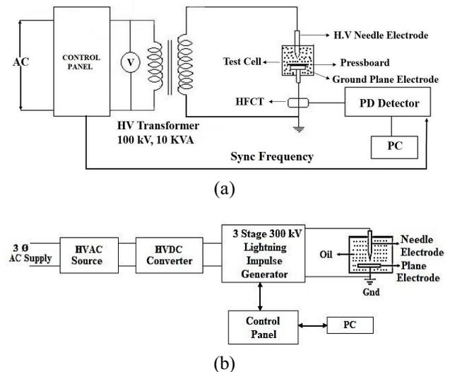
**Fig. 1.** Schematic diagram of the experimental setup for needle-plane electrode configuration (a) PD test, (b) 300 kV, 3 stage Lightning Impulse
