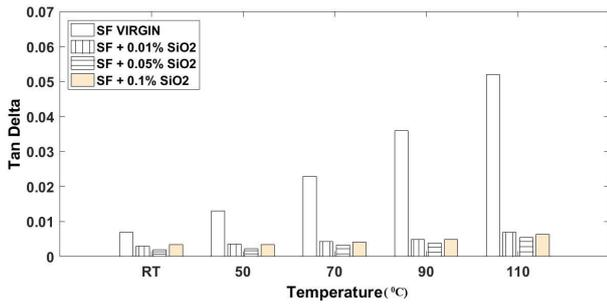
Fig. 9. Tan-Delta test for virgin sunflower oil and nano modified sunflower oil at different temperature
