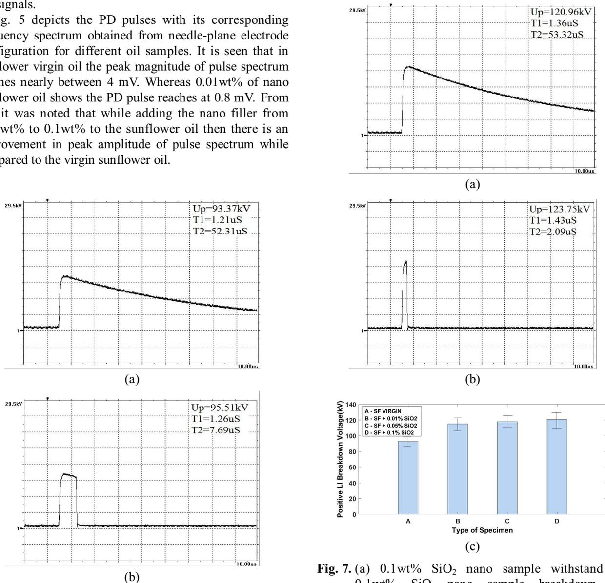
Fig. 6. Positive LI waveform (a) Virgin oil withstand (b) Virgin oil breakdown
