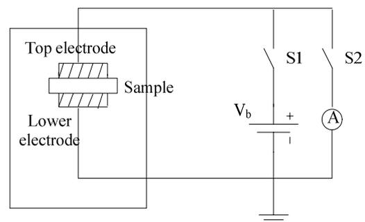
Fig. 3 TSC test principle
