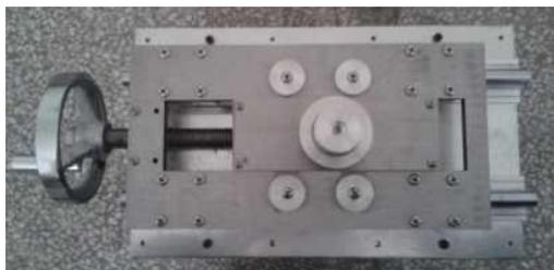
Fig. 1 Special slicing instrument for composite insulators
