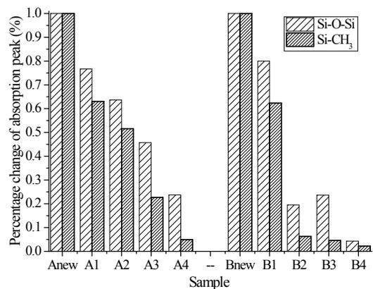
Fig. 8 Comparison of FTIR absorption peak areas
