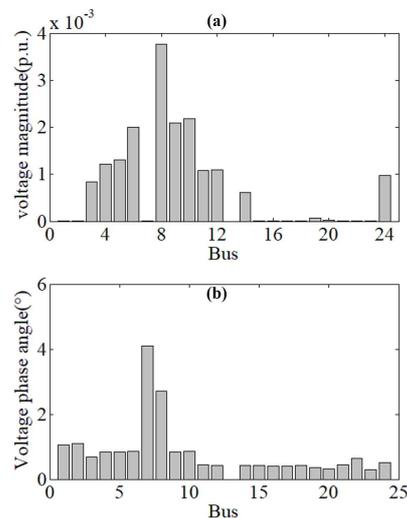
**Fig. 5.** Maximum differences of the expectations of bus voltage magnitude and phase angle between scenario A and scenario C
