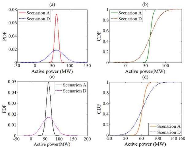
Fig. 6. PDF and CDF curves of the active power output of the slack bus
