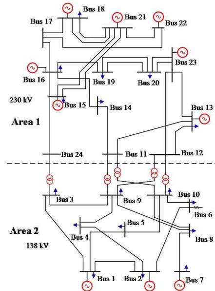
Fig. 2. The diagram of IEEE RTS 24-bus system
