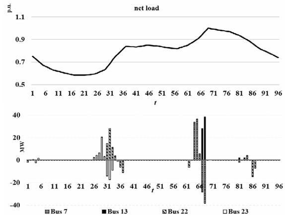
**Fig. 4.** Differences of the scheduled active power outputs of generation buses between scenario A and scenario C
