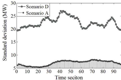
Fig. 7. Standard deviation of the active power output of the slack bus
