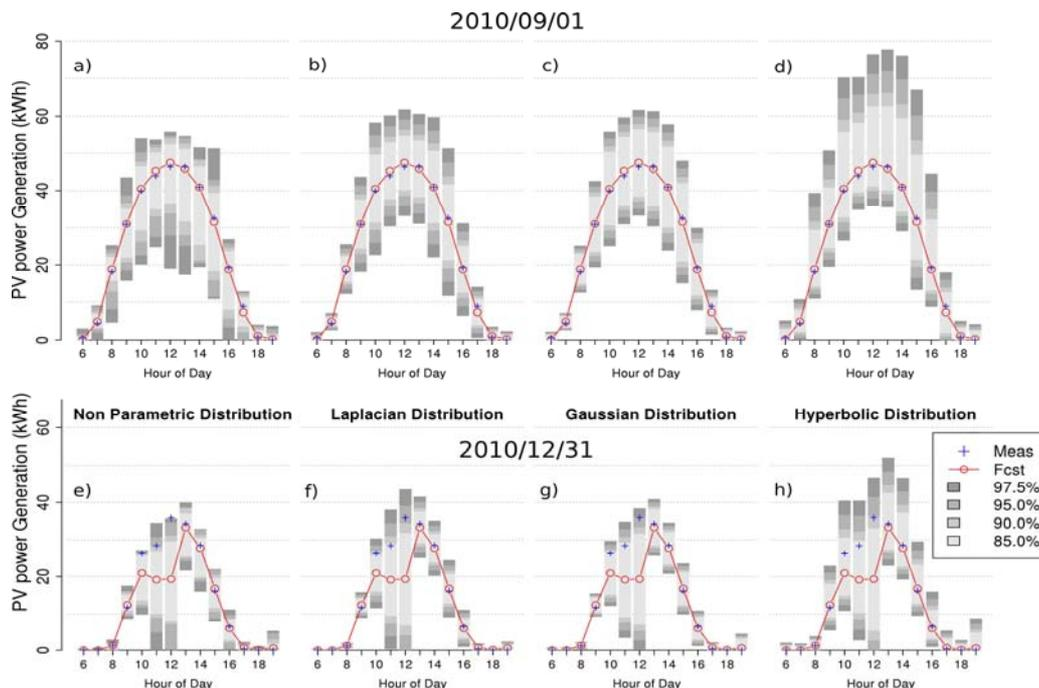
**Fig. 4.** Prediction intervals calculated (with different distribution assumptions) for two days of PV power forecasts of a single system. (Forecast error distributions: a), e): non-parametric; b), f): Laplacian; c), g): Gaussian, d), h): Hyperbolic)
