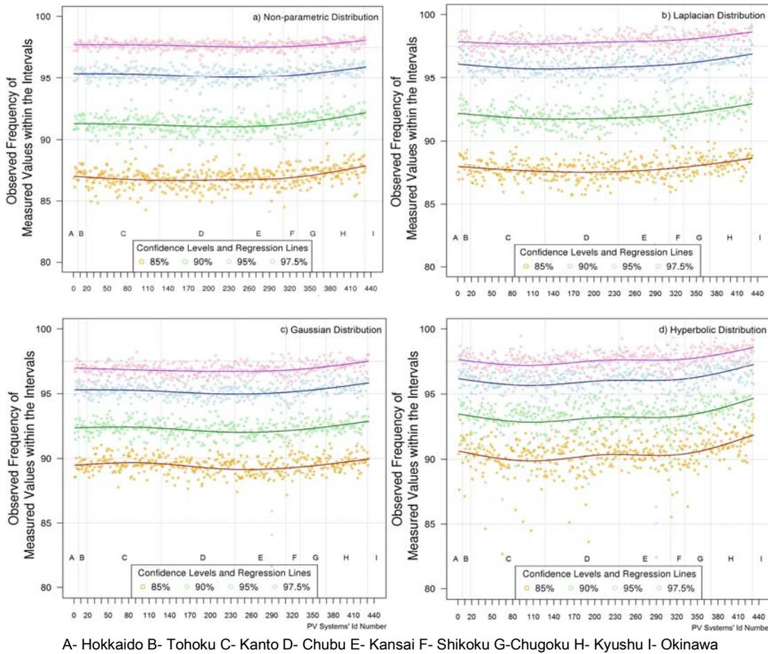
**Fig. 2.** Observed frequency of measured PV power generation within the prediction intervals (forecast error coverage) calculated with the Non-parametric (a), Laplacian (b), Gaussian (c), Hyperbolic (d) distributions from Hokkaido to Okinawa
