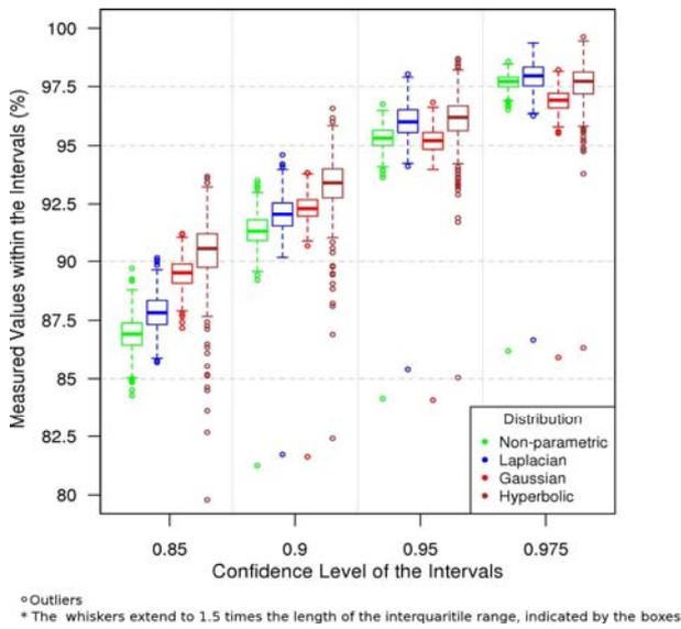
**Fig. 1.** Observed frequency of measured PV power generation within the prediction intervals for 432 PV systems, 1 year of data, and 4 confidence levels
