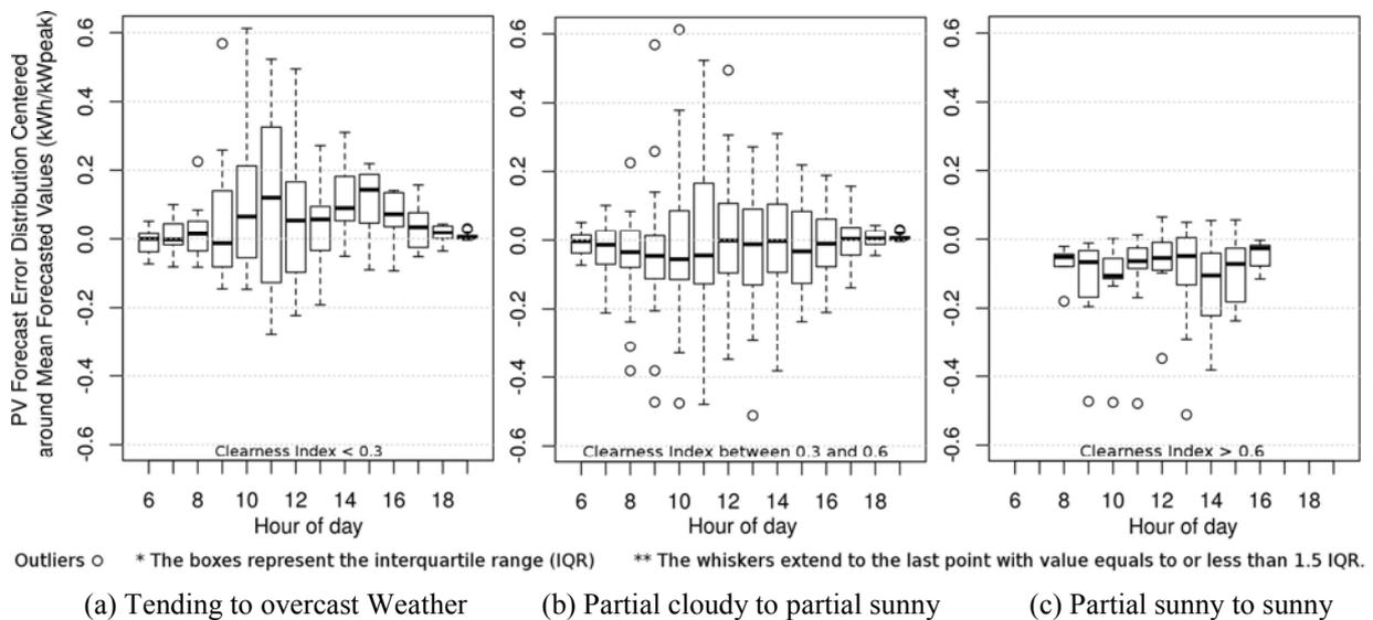
Fig. 5. Hourly distribution of the forecast error for 3 kinds of days in June of a residential PV system (10 kW<sub>rated</sub>)
