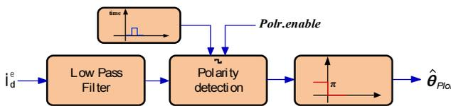
**Fig. 4.** Proposed magnet polarity detection at the initial drive startup
