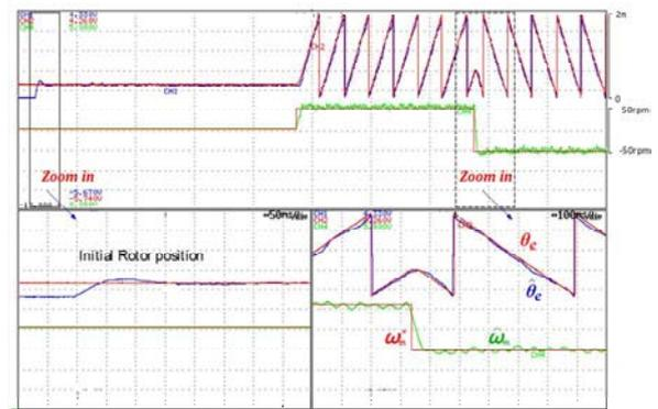
Fig. 12. Operation of the proposed method for initial rotor position and for 0, ± 50 rpm as a speed reference
