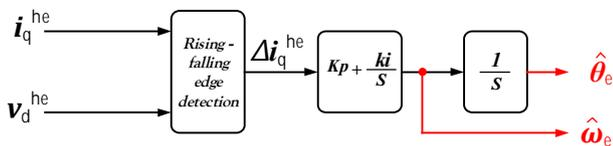
**Fig. 3.** Electrical rotor position and speed estimation based on the proposed method
