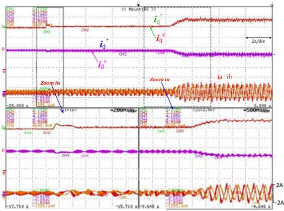
Fig.15. d-q axis current with MTPA strategy when the load is gradually increased
