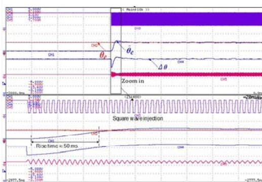
(b) Initial rotor position estimation using proposed HF square wave injection
