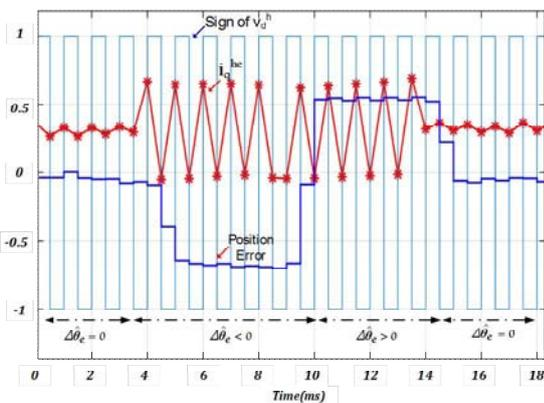
Fig. 6. Production of the position error function using the differentiation of the induced q-axis current
