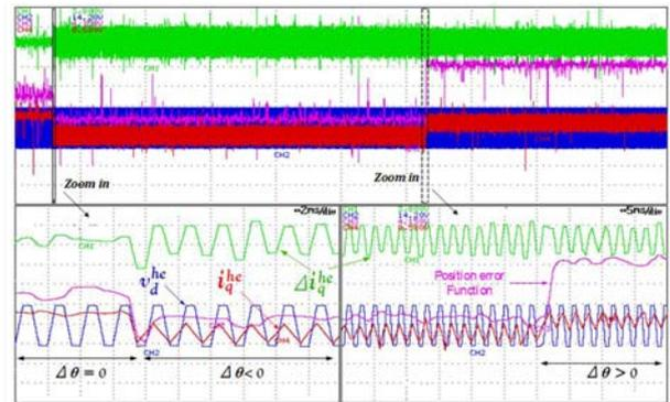
**Fig. 9.** Experimental result of the proposed method: production of the position error function
