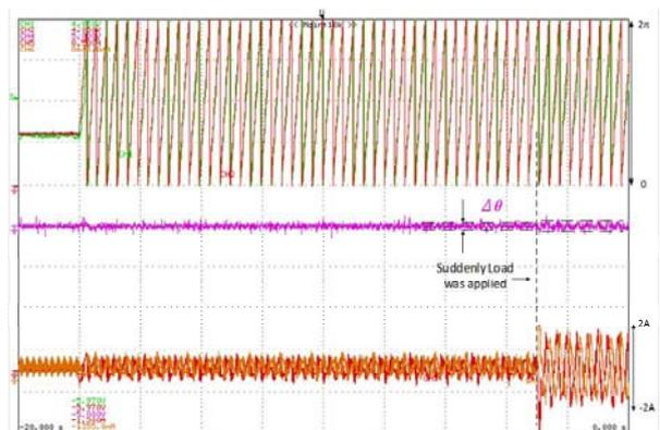
Fig. 14. Estimated rotor position, position error and phases current with and without load
