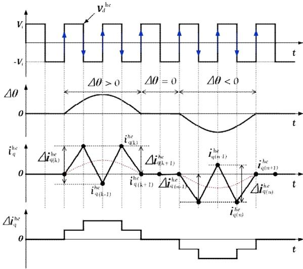
Fig. 2. Injection voltage on d-axis and resultant current on q-axis
