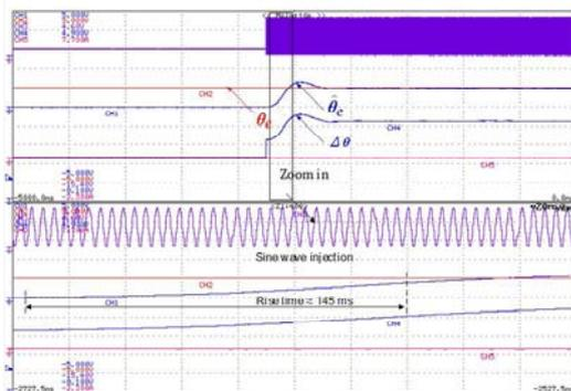
(a) Initial rotor position estimation using HF sine wave
