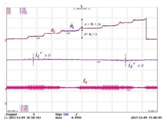
**Fig. 10.** Magnet polarity detection using the carrier d-axis current
