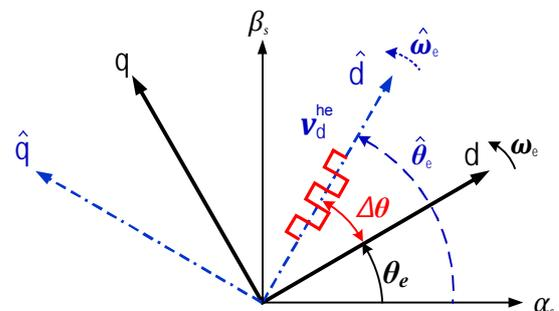
Fig. 1. Coordinate reference frame for HF pulsating square wave injection in the estimated synchronous reference frame
