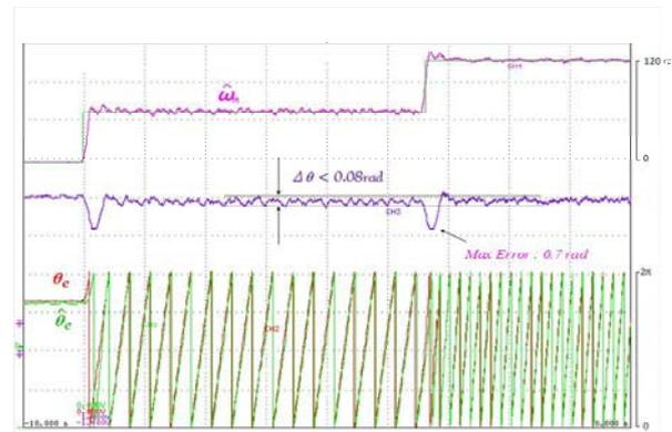
Fig. 13. Rotor position error, when the speed reference is increasing from 0, 60, 120 rpm
