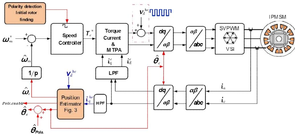
Fig. 5. Overall block diagram of the square wave voltage injection method for IPMSM sensorless drive
