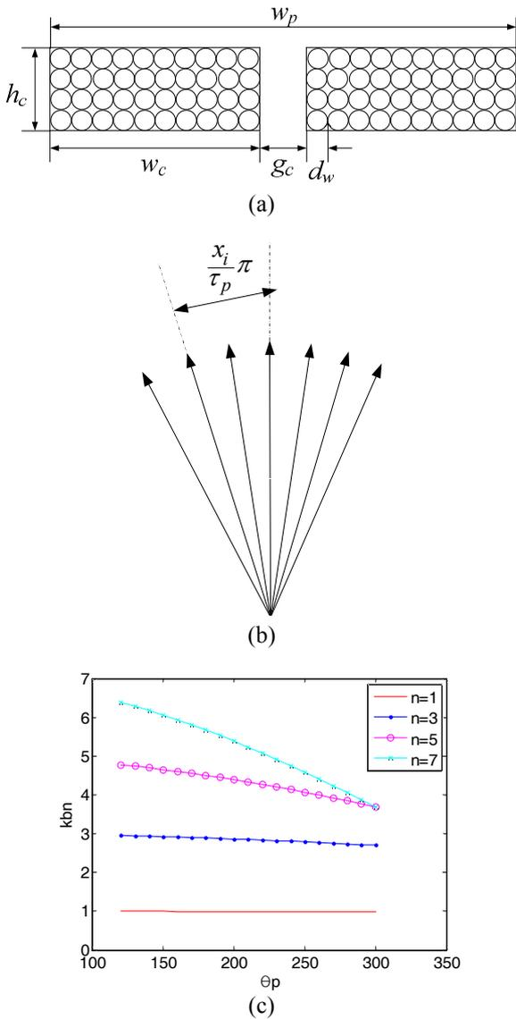
**Fig. 4.** Structure of coreless winding, (a) single concentrated winding, (b) single conductor EFM vector diagram, (c) band factor
