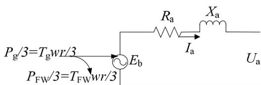
Fig. 6. Equivalent circuit for one phase of the AFPMSGa
