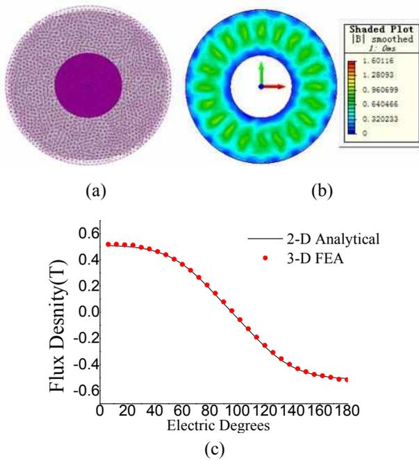
Fig. 9. (a) 3-D FEA mesh profiles, (b) flux density nephogram, (c) comparison of analytical results with 3-D FE results
