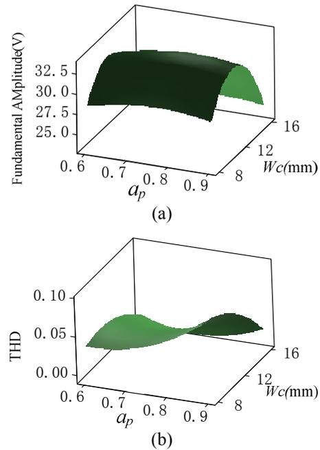
Fig. 7. RSM for polar arc and side width, (a) back EMF, (b) THD
