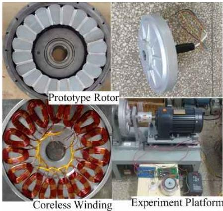
Fig. 8. Prototype machine and its main components
