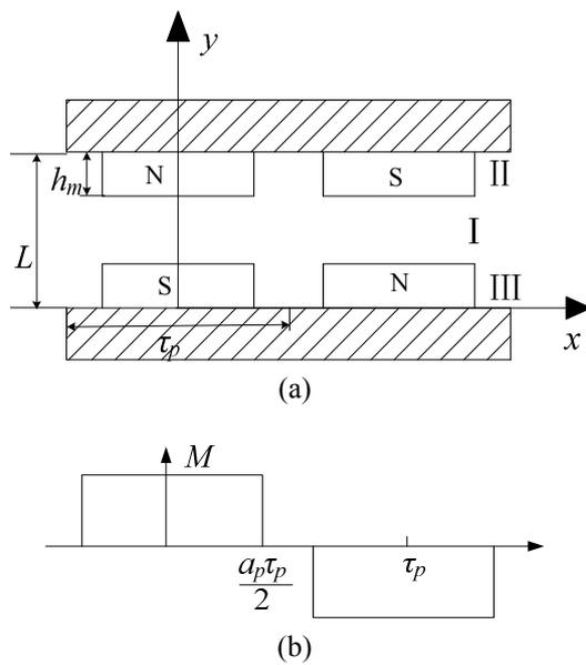
**Fig. 3.** 2-D Magnetic field analysis model, (a) Layered model (b) PM magnetization
