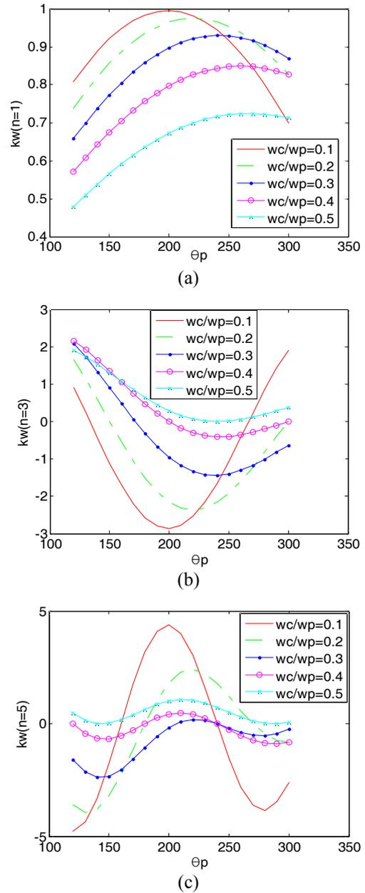
**Fig. 5.** Winding factor for different harmonics, (a)  $n=1$ , (b)  $n=3$ , (c)  $n=5$ , (d)  $n=7$
