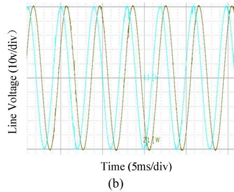
Fig. 10. No-load characteristic of generator, (a) comparison of three calculation methods, (b) measurements
