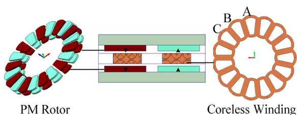
Fig. 1. AFPMSG with coreless stator windings
