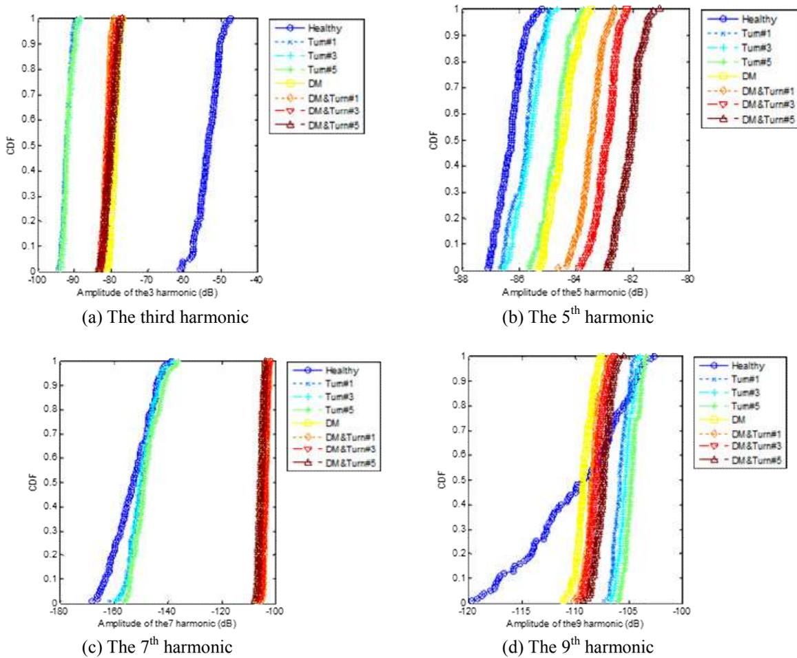
Fig. 5. CDFs of amplitudes of fault harmonics operating at 300 rpm
