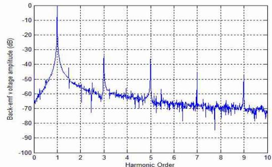
(c) Motor with demagnetization
