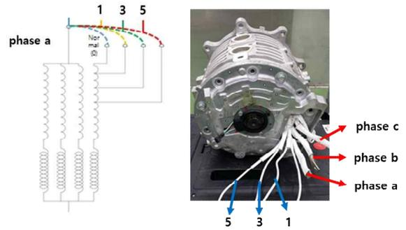
Fig. 2. Test motor with short-circuited turns
