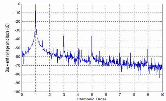
(d) Motor with multiple combined faults with demagnetization and 1 short-circuited turn
