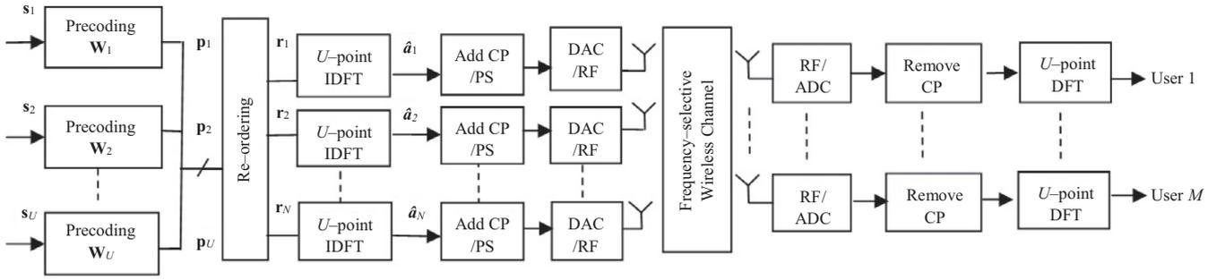
**FIGURE 1** Massive multiuser MIMO-OFDM downlink scenario, with  $U$  OFDM tones,  $N$  transmit antennas, and  $M$  user-terminals
