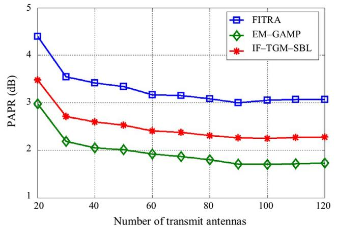
**FIGURE 6** PAPR performance of FITRA and IF-TGM-SBL algorithms vs. number of transmit antennas for  $M = 10$  and regularization parameter  $\lambda = 0.25$  for FITRA
