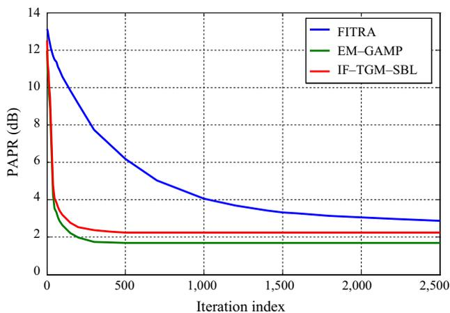
**FIGURE 5** Comparison of the convergence rates of the PAPR metric for FITRA and IF-TGM-SBL algorithms for  $(N, M) = (100, 10)$
