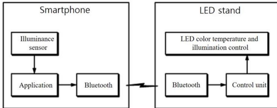
**Figure 3. Smart LED Stand Block Diagram**
