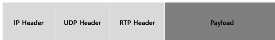
**Figure 1. RTP Packet Format**
