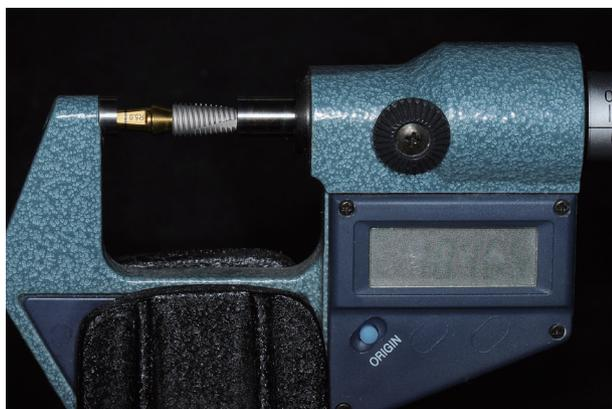
**Fig. 3.** Measurement of axial displacement.
