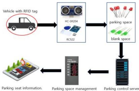
Figure 2 : Intelligence Parking Lot Control System Diagram
