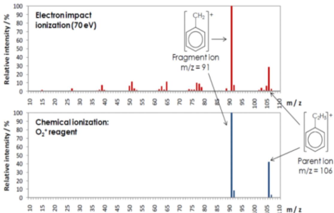
**Figure 3:** Comparison of Conventional MS Analysis and SIFT-MS Analysis
