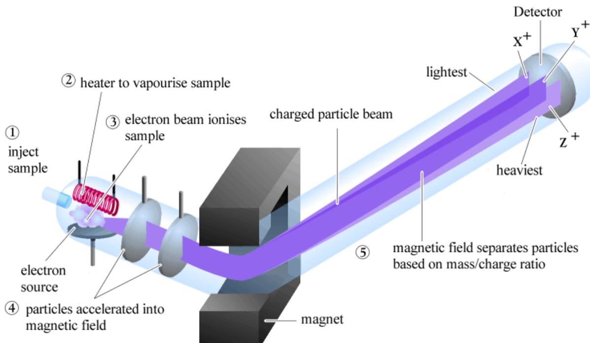
Figure 1: Mass Spectrometer Structure
