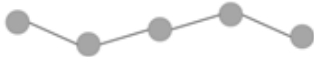
Figure 1. The cloth is modeled by a list of balls connected by rubber band.
