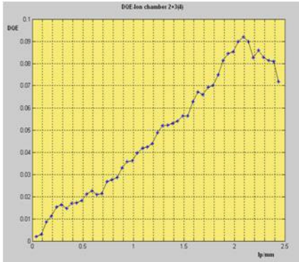
Fig. 6. Result of DQE (2+3 Ion chamber)
