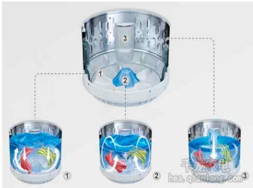
Figure 12. The schematic diagram of Little Swan "Water Magic Cube" washing machine.
