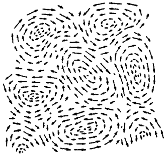
Fig.3. Proposed two-dimensional array of magnetization distributions in the ultra-soft film with nanometer scale heterogeneous structures.
