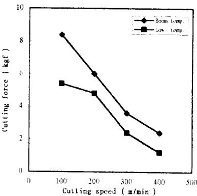
Fig.6 Relation of cutting speed(m/min) and tangential force(kgf) due to room and low temp.
