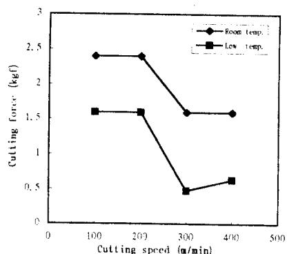
Fig.8 Relation of cutting speed(m/min) and radial force(kgf) due to room and low temp.
