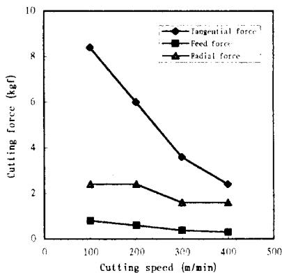
Fig. 9 Relation of cutting speed (m/min) and cutting force (kgf) due to room temp.
