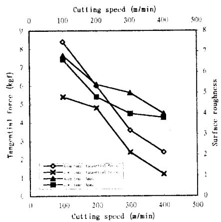
Fig. 12 Relation of tangential force and surface roughness due to room and low temp.
