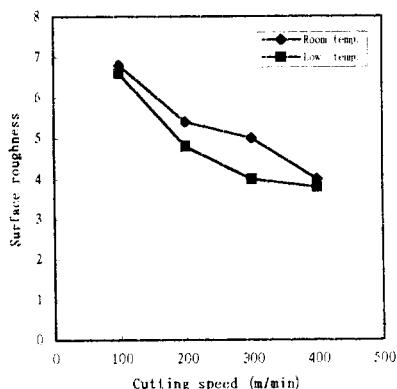
Fig. 11 Relation of cutting speed (m/min) and surface roughness due to room and low temp.
