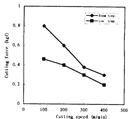
Fig.7 Relation of cutting speed(m/min) and feed force(kgf) due to room and low temp.
