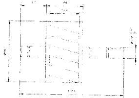
Fig.4 Dimension of cage motor rotor
