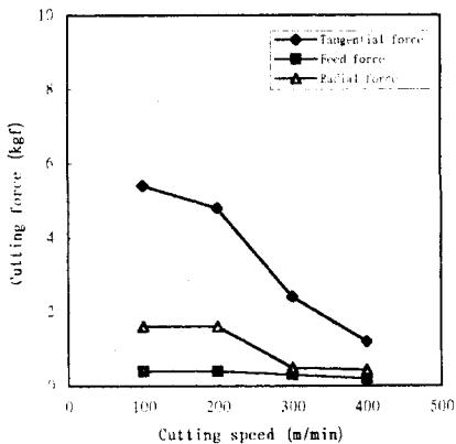
Fig. 10 Relation of cutting speed (m/min) and cutting force (kgf) due to low temp.
