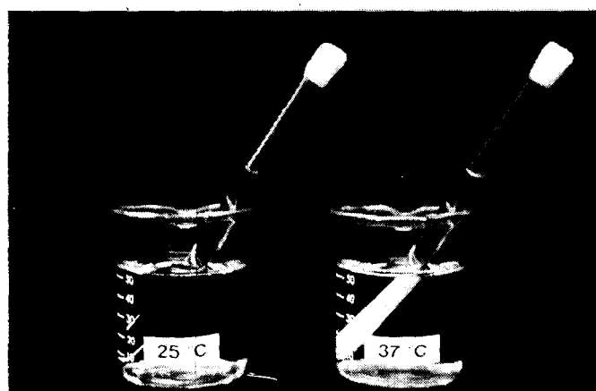
Figure 1. Thermo-responsiveness of PNIPAAm. 1.0 (w/v)% aqueous solution of PNIPAAm prepared below the LCST is insoluble and forms a precipitate at the cell culture temperature of 37 °C, however becomes instantly soluble in water at room temperature. This change from a soluble state to an insoluble state is reversible below and above the LCST of approximately 31.8 °C. The conversion is caused by the temperature-dependent formation and destruction of hydrogen bonds between the water molecules and the amide groups of the PNIPAAm.
