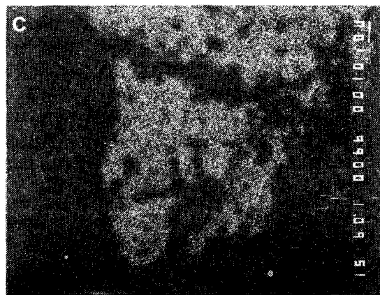
Fig. 2. Microphotographs of X-ray emission images for alkali-quartz reaction. A: The same site as the square illustrated in Fig. 3A, B: K distribution; C: Na distribution; D: Si distribution.
