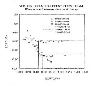
Fig.2 Flooding map with steady air flow
