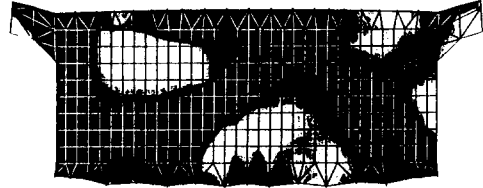
Fig. 2 Optimal topology of package tray
