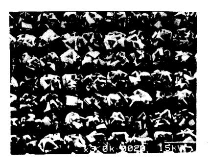
FIG.1. SEM Micrograph of the patterned diamond rods
