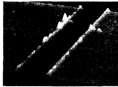
Fig. 6 AFM image of grooved edge by C3M (Load 95.7mN, Feed rate 150 \mu m/s)
