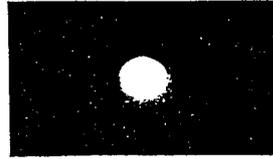
Mode profile of channel waveguide
