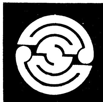
Fig.14 Electrical discharge machined SiC-ZrB<sub>2</sub> 30Vol.% composites
