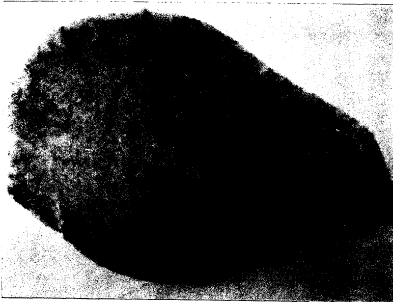
Fig. 1. An electron micrograph of the thin section of a fine ZnO particle.
