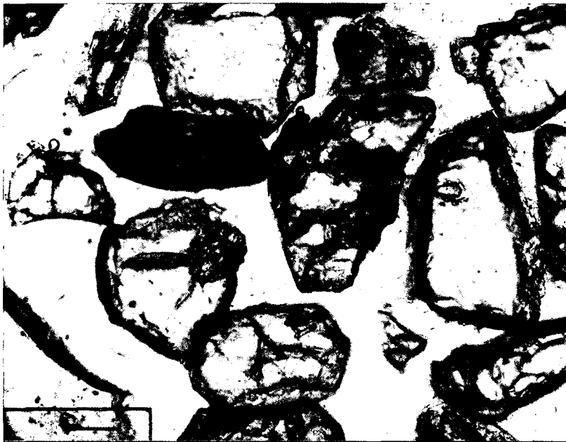
Fig. 1. Polarizing micrograph of garnet powders of homogeneous size prepared by a vacuum embedding method. (scale bar: 0.1mm)
