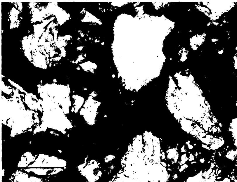
Fig. 2. Polarizing micrograph of garnet powders of heterogeneous size prepared by a centrifuging method. (scale bar: 0.1mm)
