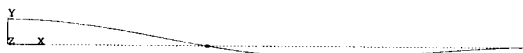
Fig. 2. Mode shape of a circular plate for nodal circle m = 1 and nodal diameter n = 0 .
