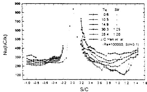
Fig. 7 Nusselt number distribution on the blade surface
