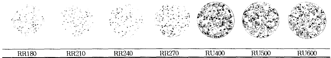
Fig.1 Coarse aggregate content ratio obtained by Volumetric Area Method
