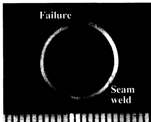
Fig. 3 Macrostructure of failure tubular heating element by bulging
