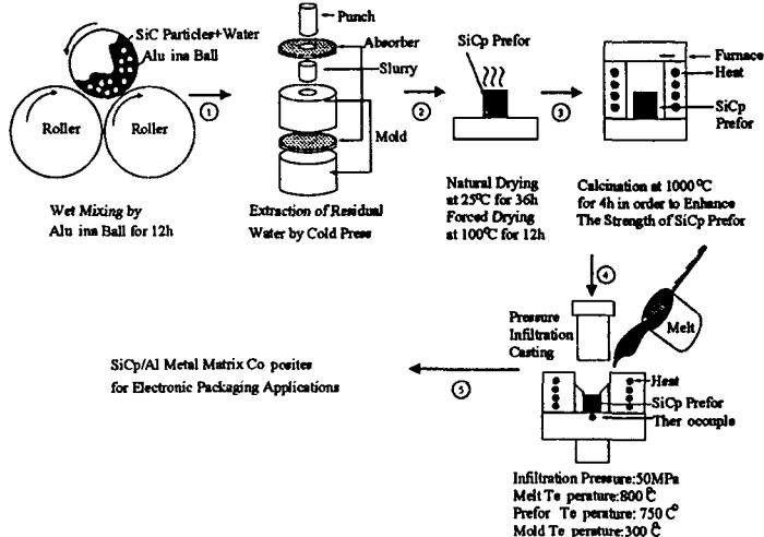
Fig. 1. Fabrication process of high volume fraction SiCp/Al metal matrix composites by pressure infiltration casting process.
