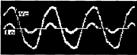
Fig. 12 Experimental result of output waveforms ( V_c, I_o ) with rectifier load. (20 V/div, 20A/div)
