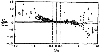
Figure 1. Variation of eddy viscosity coefficient with curvature parameter S_c . open symbols: present data closed symbols: data of Holloway and Tavoularis(1992)
