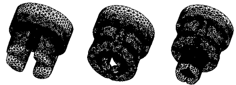
(a) Divding (b) Welding (c)Forming Fig. 2 Extrusion stages of porthole die
