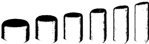
Fig. 1 Intermediate cup shapes for the original design
