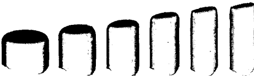
Fig. 2 Intermediate cup shapes for the modified design
