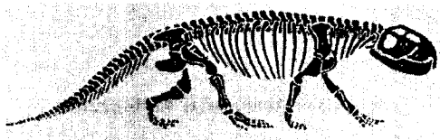
Fig. 1 Model of Terrestrial Vertebrate for the 4-Legged Walking Machine Design.
