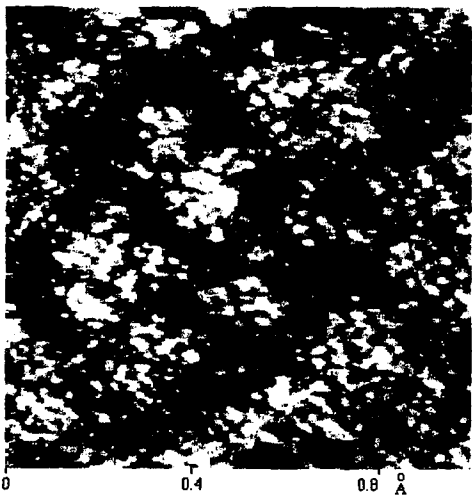
Fig. 1. AFM image of La-Sr-Mn-O thin film at OMR 0.17
