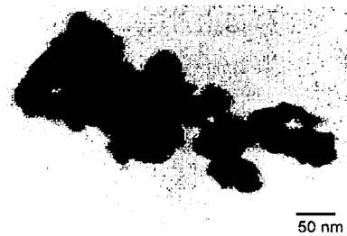
Fig. 2. The TEM images of Ni_{0.63}Zn_{0.17}Cu_{0.2}Fe_2O_4 powder annealed at 400 °C .
