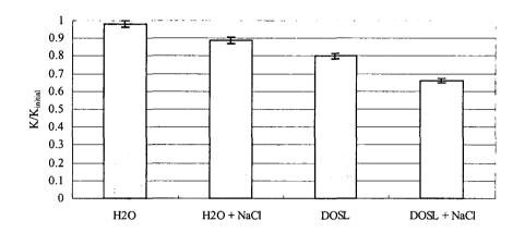
Fig. 1 Fraction of hydraulic conductivity relative to initial values after leaching with three pore volumes of control or surfactant solutions
