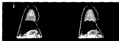
Fig.3 biprism image of molten pool surface
