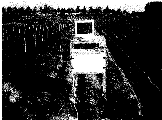
Fig. 3 Mobile platform with vision system
