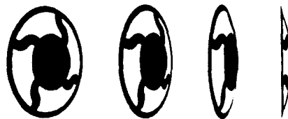
Fig. 7. Opening postures of CSF shunt valve from different angle of views
