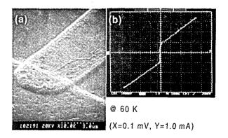
milling to define the junction width. Finally, Au was also deposited by PLD and patterned by lift-off for the contact pads.
