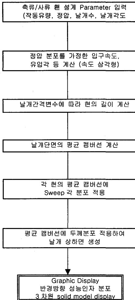
Fig. 1 Flow chart for fan design
